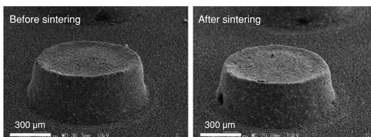
Figure 3 Shape change before and after sintering
