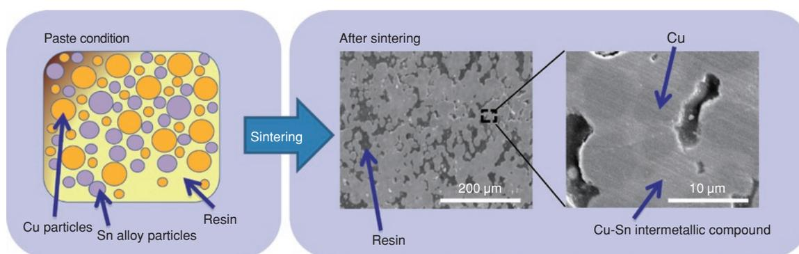
Figure 1 Structure of HT Series
